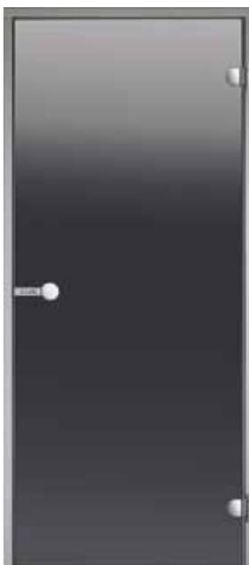
The aluminium frame door is an excellent solution for a steam room or a sauna door. It is designed for conditions where the materials need very good humidity resistance. There are no wooden parts in the door. The aluminium frames (40 x 60 mm) are light grey in colour. The glass is tempered 8 mm safety glass. Seals keep the heat and steam in. Aluminium frame door is maintenance-free decade after decade.
